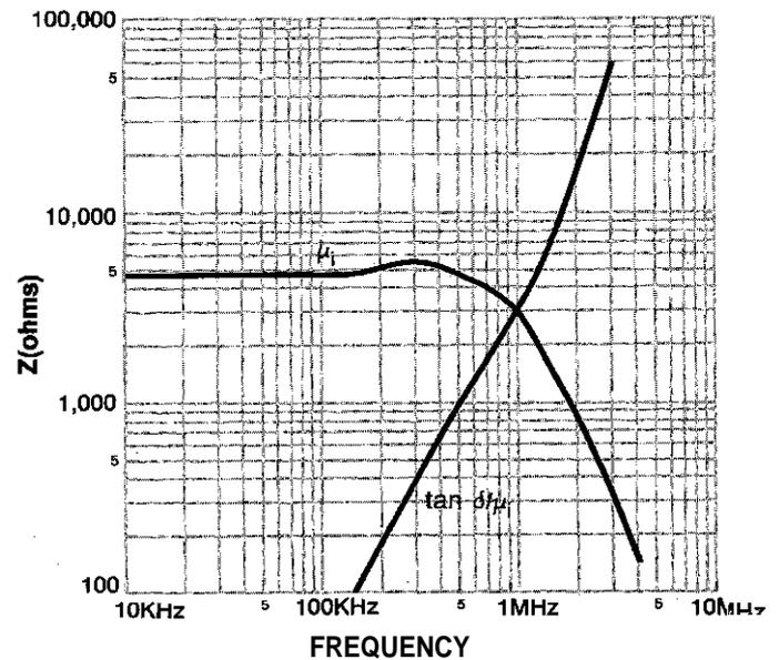
loss factor increasing with frequency causes the resistance to ultimately become the dominant source of impedance at high frequencies.
