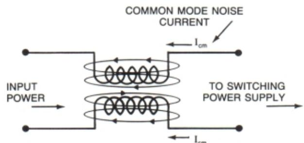
generated in the core which cancel each other and thus almost no voltage is induced in either winding. The input current needed to power the SMPS therefore will pass through the filter without any appreciable power loss.
